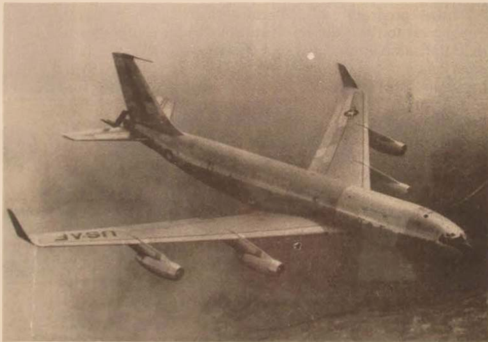
Not to be forgotten is the KC-135 Stratotanker (left), also undergoing wing modifications to stretch its operational lifetime into the 1990s. This tanker was chosen because its wings can be easily modified, and the test results can be readily applied to other transport-class aircraft. . . . Artist's concept of an Air Force KC-135 testbed aircraft with winglets on the outer wings (above). Flight testing of winglets on a KC-135 is scheduled to begin late in 1978. Wind tunnel tests indicate that significant fuel savings can be had by transport-class planes with the winglets.
